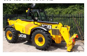
Max lift capacity **3,500kg**Max lift height **12,070mm**Max forward reach **8,060mm**Capacity at maximum reach **1,150kg**Engine power gross **75hp(55kW)**
